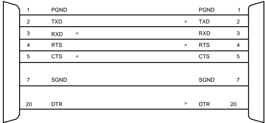
Figure 2 - Model 24 (DTE) to DCE Device
