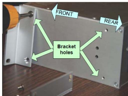
Attach brackets and unit to rack with four screws as shown below.
