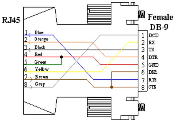
Use with RJ08X007 Cable only if controller has a B/C and is set to "C")
