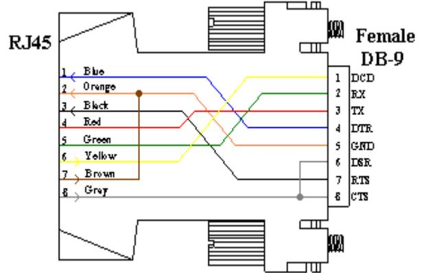
Use with RJ08X007 Cable Without B/C switch or With B/C switch set to "B")
