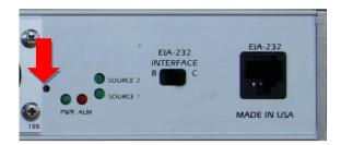
NOTE: ATS units after 2018 do not have (B/C) switch On the front panel is a small hole next to the LED, similar to the above picture. Perform the following steps:
